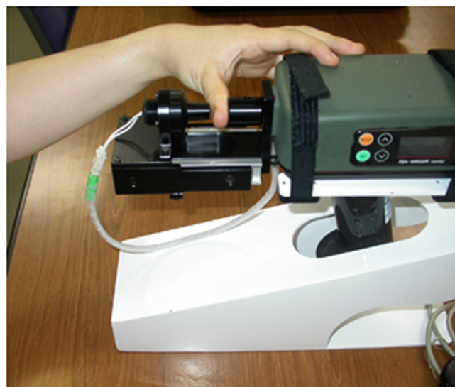
Fig. 1. Spectrophotometer used for collection of Vis-NIR spectra. Vis-NIR spectra collected from the thumb by FQA-NIRGUN spectrophotometer were used for the potential diagnosis of CFS.
